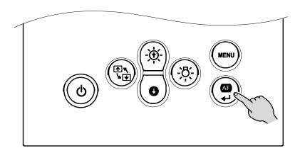
The auto focus can also be performed by pressing the AF button in the camera head.
