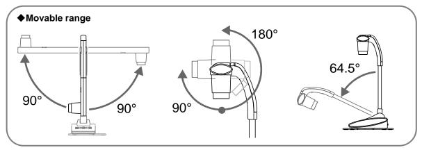
Depending on the position of the camera head or the installation place of the LX-1, stable operation may not be possible. In that case, change the position of the base plate.
