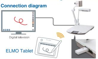
The CRA-1's wireless adapter can be plugged into the P30HD directly, allowing direct annotation on live images from anywhere in the room without using a computer.
